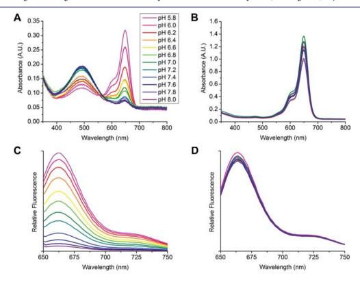
Figure 2. Spectral properties of cyanine-PFPE conjugates in phosphate buffers. Inset (A) shows pH range for series. Absorbance spectra (A) of CypHer5-PFPE oil (14, 17, and 18) and (B) Cy5-PFPE oil (13, 16, and 18). Fluorescence emission spectra of CypHer5-PFPE (C) and Cy5-PFPE (D) nanoemulsions 22 and 21, respectively. Excitation wavelength was 630 nm.
