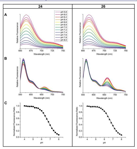
**Figure 3.** Fluorescence spectra and pH response of ratiometric nanoemulsions **24** and **26** in phosphate buffers. Inset (A) shows pH range for series. Emission scans ex 630 nm (A) and em 530 nm (B). pH-ratio calibration curves (C) normalized to maximum fluorescence ratio value (at pH 4.0), averaged from synchronous and fixed wavelength scanning methods. pK<sub>3</sub> of both formulations is 6.8.
